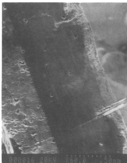
Fig. 17. SEM/XES graph of an air cathode cross section after 1 h operation in 12 N KOH ( 100 \text{ mA cm}^{-2} , 65 \text{ }^\circ\text{C} ). Tracing element: potassium.
