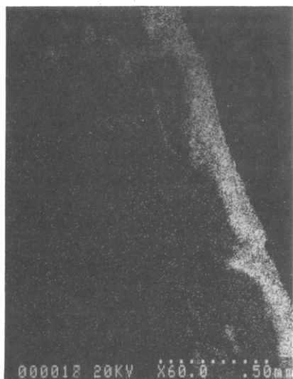
Fig. 19. XES graph of an air cathode cross section after 217 h operation in 12 N KOH ( 100 \text{ mA cm}^{-2} , 65 \text{ }^\circ\text{C} ). Tracing element: potassium.
