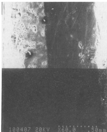
Fig. 17. SEM/XES graph of an air cathode cross section after 1 h operation in 12 N KOH ( 100 \text{ mA cm}^{-2} , 65 \text{ }^\circ\text{C} ). Tracing element: potassium.
